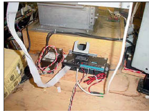
Picture 3: The Coin Tech Game System 'kit' installs easily into any game. We found it much easier to Velcro the small computer board inside of the game's cashbox but for our first install, we wanted to be able to quickly convert the entire game room back to tokens in case the system and its back-up went down (which it has not).
